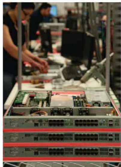
Visual inspection work centers are dedicated to performing physical assembly inspections for every build. Source: MBX Systems
