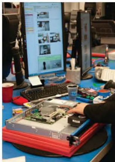
Visual build documents displayed at the relevant work center assure assembly accuracy. Source: MBX Systems
