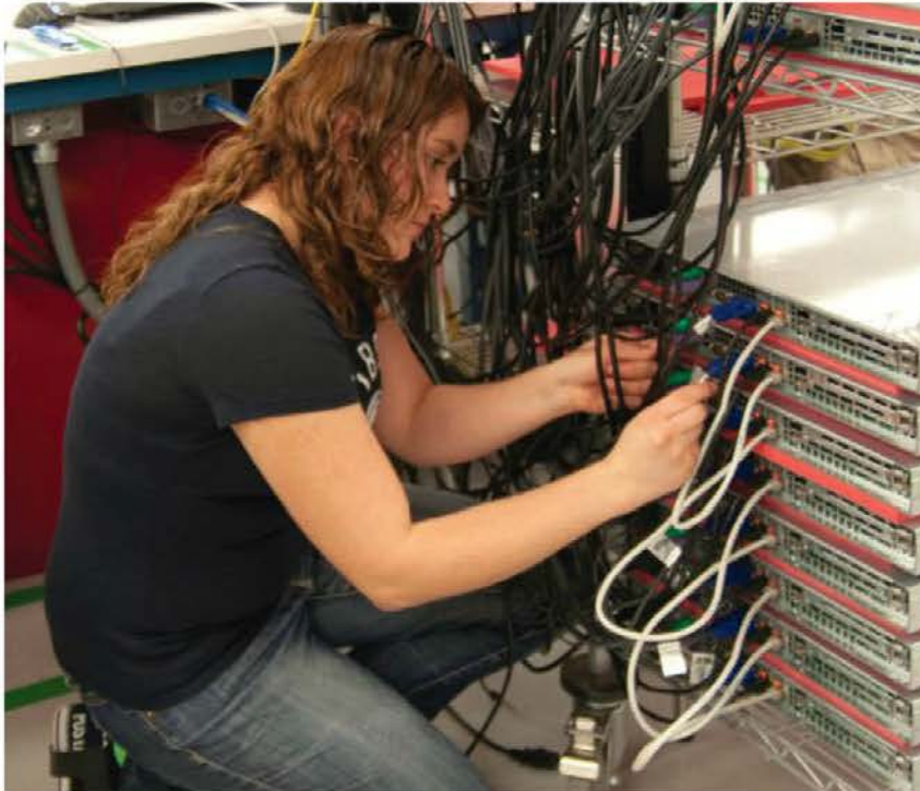
Quality control technicians conduct routine and custom functionality testing after physical inspection. Source: MBX Systems
